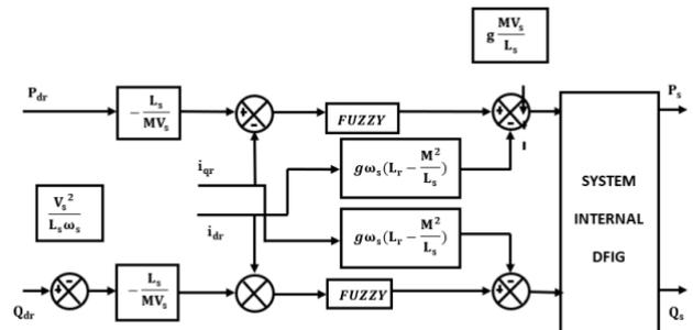
Fig.9. Block diagram of the FLC structure.
