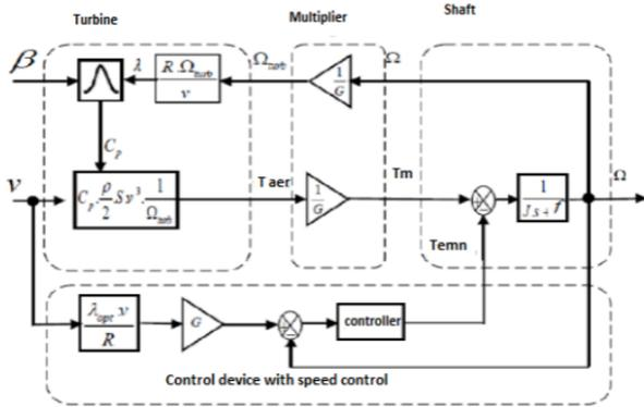
**Fig.2.** Block schematic of power extraction maximization with speed control.
