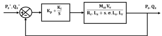
Fig.8. Block diagram of PI control structure.
