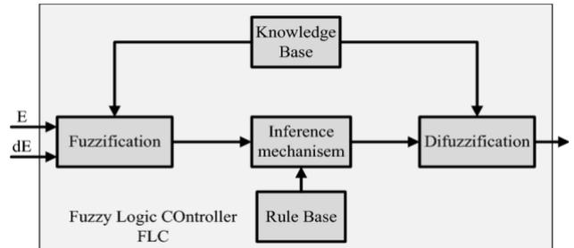
**Fig.5.** Block diagram of a FLC.
