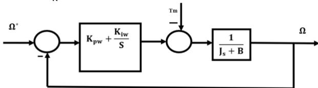
**Fig.3.** Loop diagram for speed control using a PI controller.
