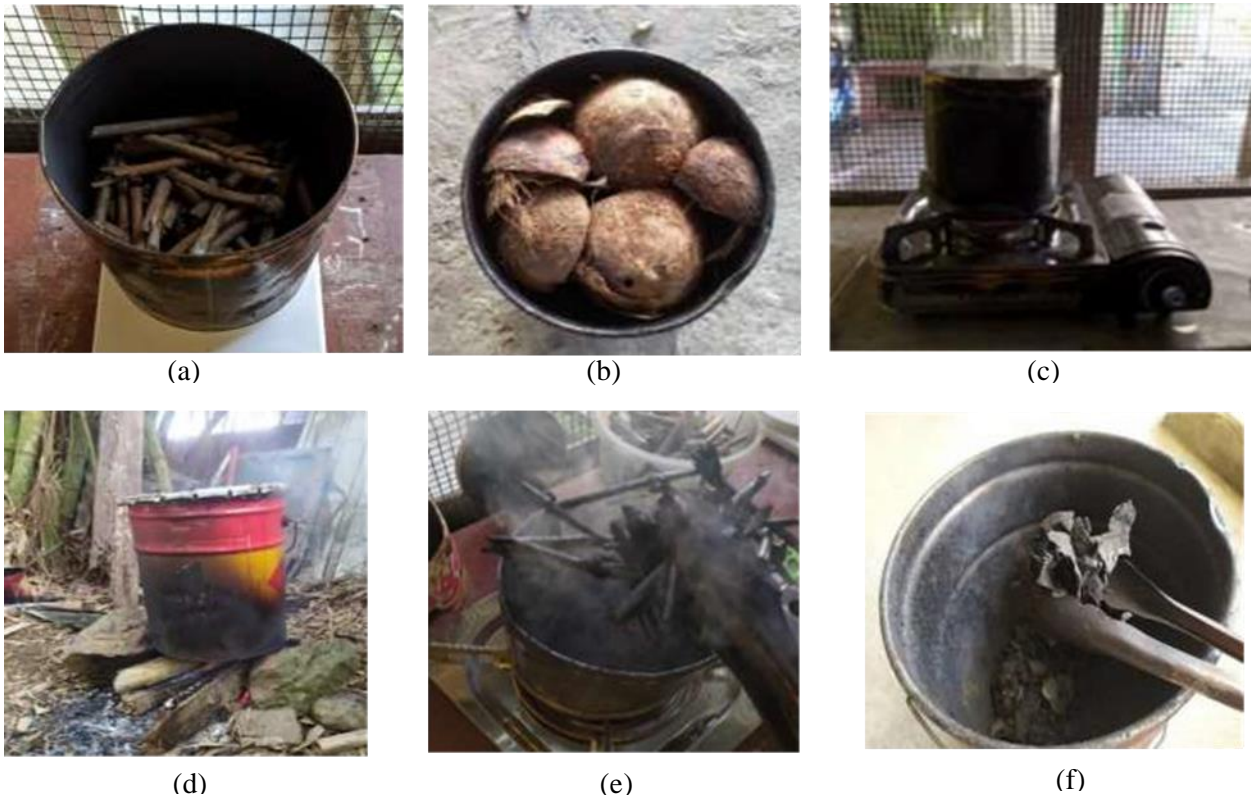
Fig 1. The process of burning raw materials from ingredients to charcoal
