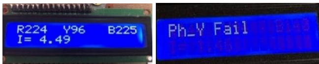
Fig. 9. When the Y-phase is missing or unbalanced.
