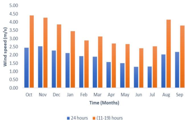
Fig. 2. Wind speed behavior in the high Andean region Average annual wind speed values recorded during October 2019 to September 2020
